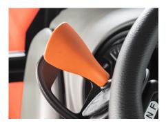
PowerShuttle Electro-hydraulic reverser
